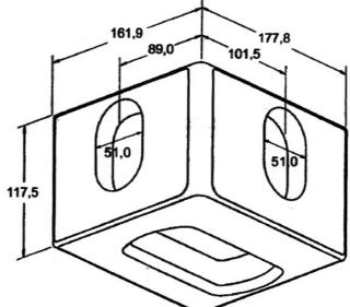
The castings are properly cast, dressed, normalized, shotblasted and machined on the outside surfaces; made of *Aldur S 45*, a non-ageing, fine-grained structural cast steel, resistant to brittle fracture with high yield strength, guaranteed weldability and designed for low temperature working (at -40°C as standard).
